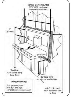
4. Place the unit into the recessed area and insert the screws and flat washers to hold the unit in place. It may be necessary to adjust the level of unit by using a shim on the top right or left side of the unit before tightening securely to the studs.
