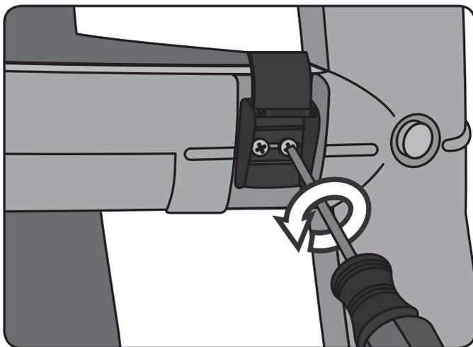
**2.** Locate the plastic clip on the left leg and open it so that the two screws securing it to the leg are exposed. Using a Phillips Head Screwdriver remove the two screws. Discard the old clip and screws.
