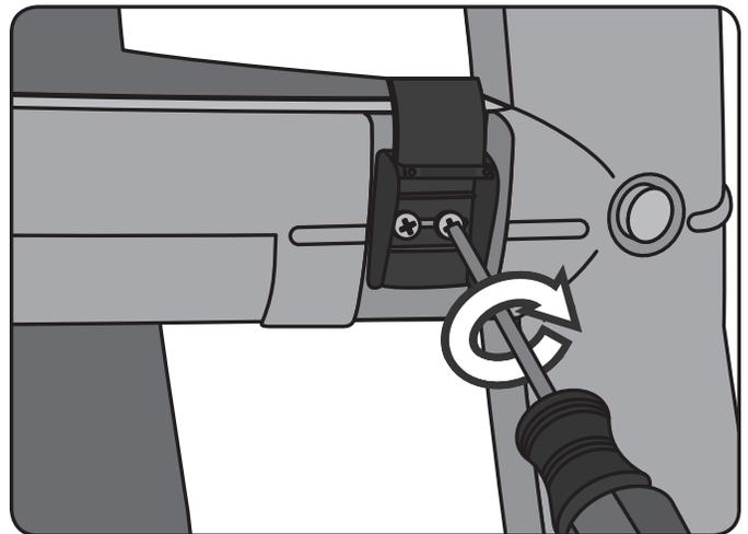
**4.** Take the new clip and position it on the left leg so that slot in the clip aligns with the two holes on the left leg. The plastic lever should be at the top of the clip. Using a Phillips Head Screwdriver, secure the clip to the leg with two of the screws provided.
