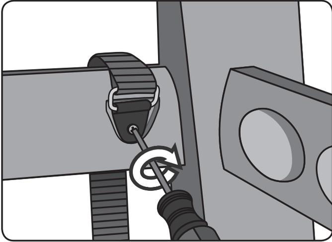
5. Take the new strap and position it on the right leg so that the hole in the chafe tab aligns with the hole in the right leg. Use a Phillips Head Screwdriver to secure the strap to the leg, using the screw provided.
