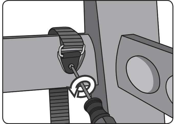
**3.** On the right leg, loosen the screw securing the strap to the chair. Discard the old strap and screw.
